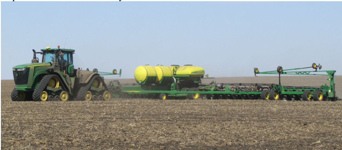
Figure 1. – This is a quad-track tractor pulling a 36-row planter with a center-fill unit (yellow container). At 90 feet wide and driving 6 miles per hour (mph), it can plant 65 acres per hour! Some 24-row planters (60 feet wide) can go 10 mph and plant 75 acres per hour (this does not include the time for end rows or putting seed in the planter).
