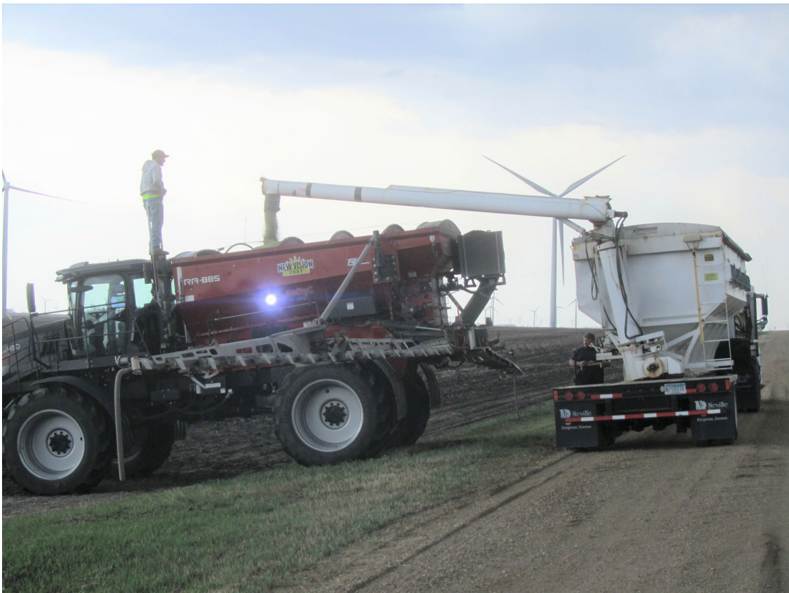
Figure 2 – This applicator is being loaded with fertilizer for a corn field in Jackson County. The tender parks on the road and augers the fertilizer onto the machine. Yes, that is the applicator driver standing on top of the machine stretching his legs and monitor the machine being filled. These applicators put in some long hours in the spring.
