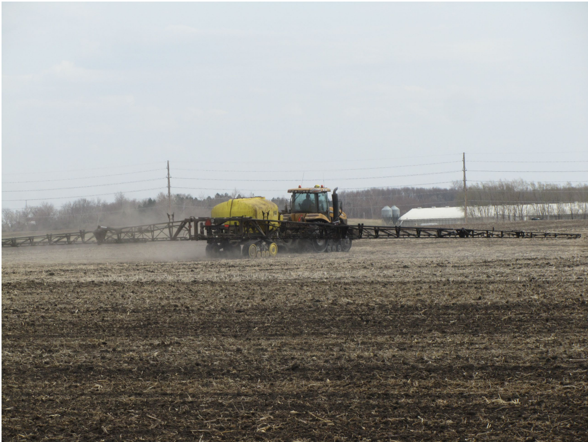
Figure 4 – This sprayer is applying liquid nitrogen just before the field cultivator tills in into the soil. The yellow tank holds about 1500 gallons and the boom is about 120 feet wide. On this unit, both the tractor and the sprayer are on tracks.
