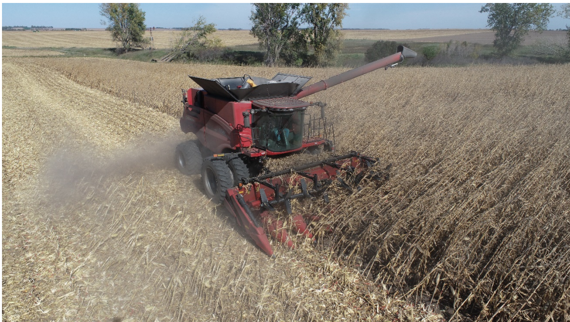
Figure 3 – Combining down corn. Some producers could only combine one direction, some could only use a portion of the head, and some had to add mechanical help like the paddles shown above, all to pick up as many ears as possible.
