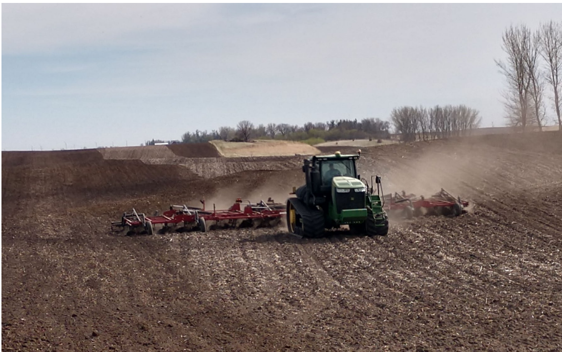
Figure 2 – This is a field cultivator in Delafield Township in Jackson County. With the Global Positioning System (GPS), the tractor is set to sub-inch accuracy so that there is very little overlap for each pass through the field, which saves time and money.
