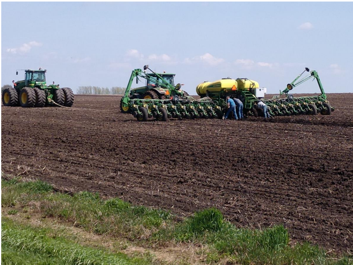
Figure 2 – This is a picture of a common occurrence this spring. The planter went down in a wet spot and had to be pulled out with the 4WD tractor on the left. You can see the producers working on cleaning the mud-filled seed drop tubes.
