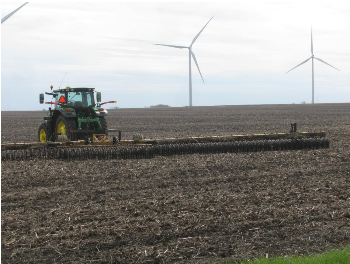
Figure 3 - This is a large rotary hoe that can be used to aid in corn emergence by breaking up soil that has become “crusty” on top, or used to help dry out soil ahead of soybean planting, especially in a ridge-till system.
