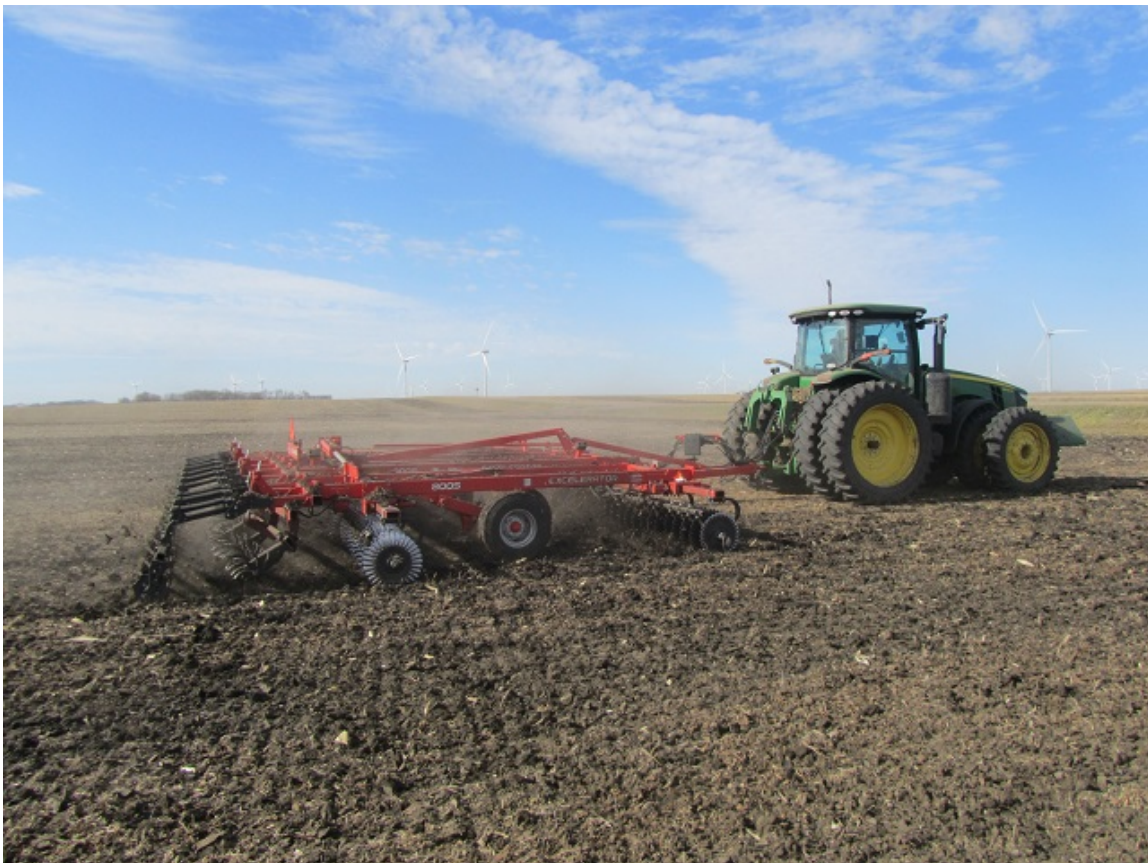
Figure 2 – This is a vertical tillage machine that is used after soybean harvest in preparation for the corn crop in 2019.
