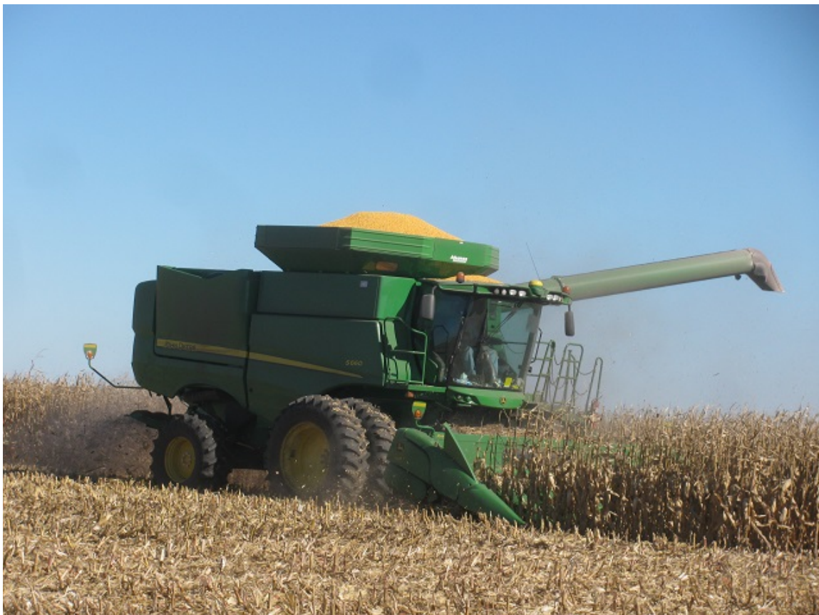
Figure 3 – These machines continue to be amazing. A combine of this size can harvest over 150 acres per day with the right field conditions and grain handling equipment.
