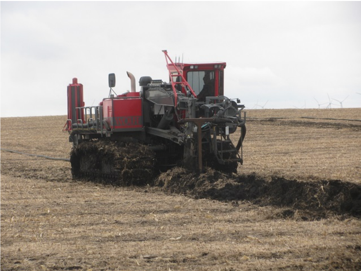
Figure 4 – As harvest concludes, we are working with several landowners to install drainage tile yet this fall. This has been another year that tile has provided significant returns to landowners.
